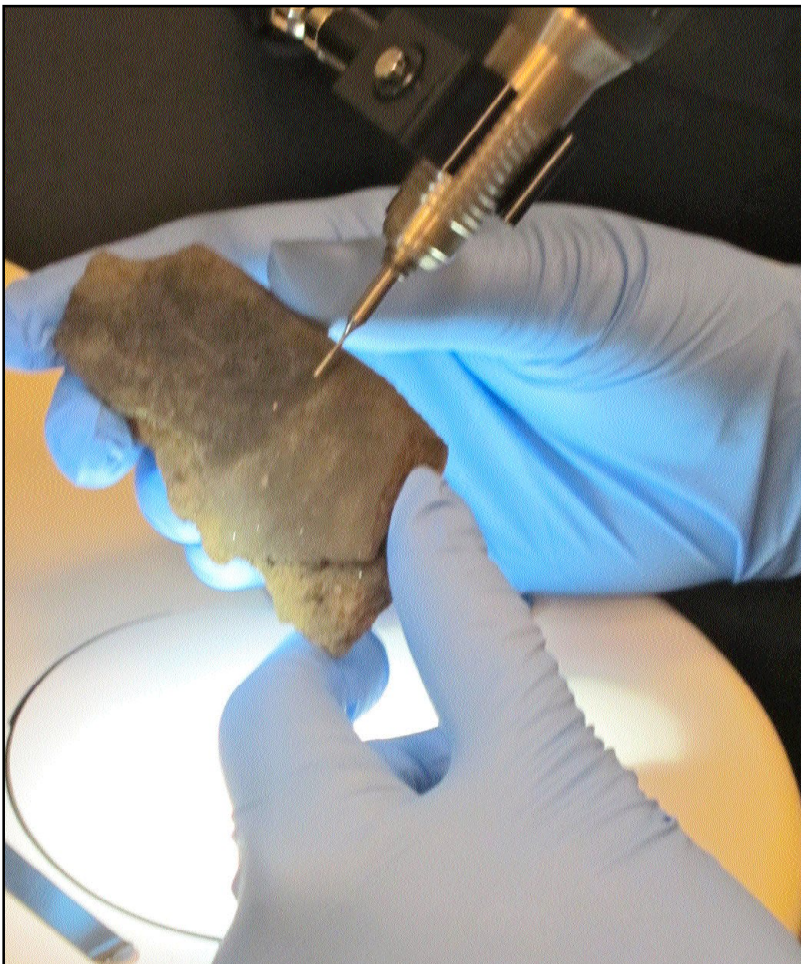
Figure 3: A silicon carbide drill bit mounted on a precision drill attached to a stereomicroscope allows research associate Meghan Burchell to remove micro-scale samples of carbonized residue from ceramics for isotope analysis. (Photo by Katherine Cook)
